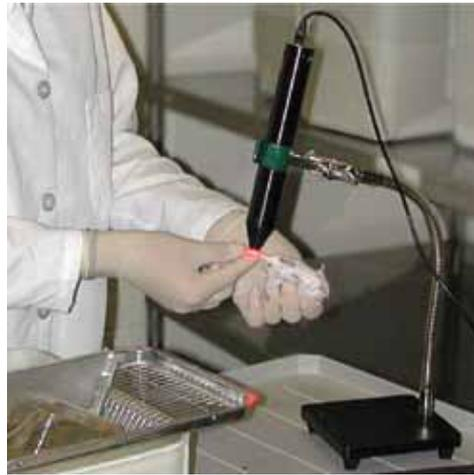
Figure 6. The set-up to tag mice. A stand with the wand is shown during the process of reading the p-Chip ID.
